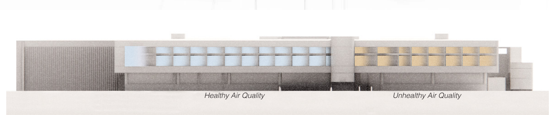
Healthy Air Quality Unhealthy Air Quality DIAGNOSTICS DISPLAY- FACADE GLOW Indicates air quality measured from rooftop weather station to the community and commuters
